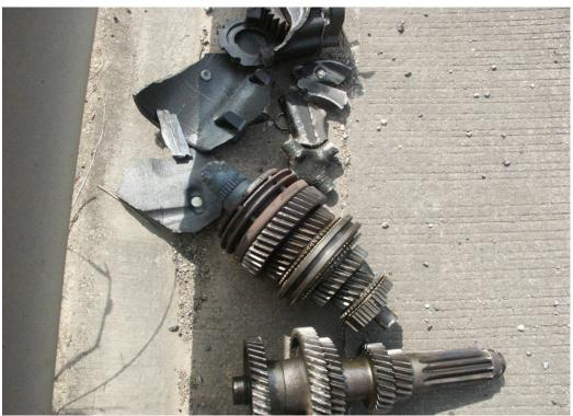
This collection of parts from a truck gear box was found on the Cockle creek overpass. The gears seen in the centre of the photograph have a fractured straight cut. The drive shaft in the top has also twisted and fractured. Its grey colour change suggests super heating. There are few traces of gear oil on the parts.
