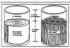
Fig. 3. Examples of suggested loading techniques for wood samples and for carpet or vinyl flooring (chimney roll).
